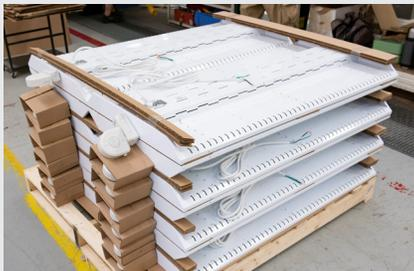
Product is layered and supported with corrugate inserts between each layer of fixtures.
