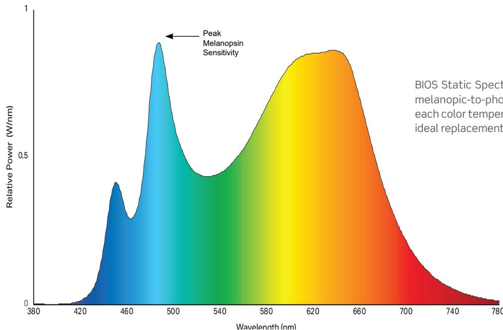
BIOS Static Spectrum Light Engine delivers the industry's best melanopic-to-photopic (M/P) ratio, with R9 greater than 90 at each color temperature. BIOS Static Spectrum Light Engine is the ideal replacement for static color light fixtures.
